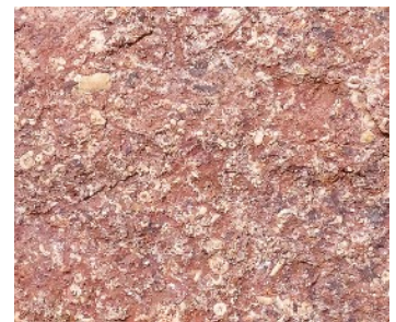
Fig. 13 Abundant crinoid ossicles in the Castle entrance wall, whole ossicles here are typically 3-10 mm diameter but most are fragmented.
